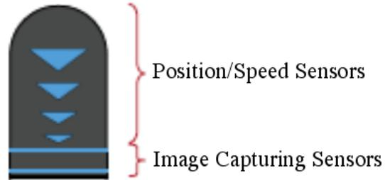
Your TimeIPS biometric fingerprint reader has several position and speed sensors that detect the contact status and swipe speed of your finger. The last sensor is the image capturing sensor that reads the fingerprint. For that reason, it is essential that you place your whole finger covering the entire surface of the sensor and maintain light pressure and a constant speed through the entire swiping process in order to get the best possible fingerprint read.
