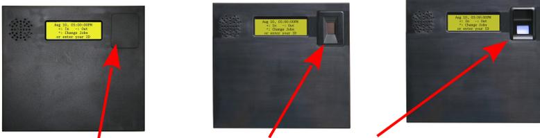
IPS125T: No biometric sensor. IPS125T-B, IPS125T-O: Biometric sensor installed
