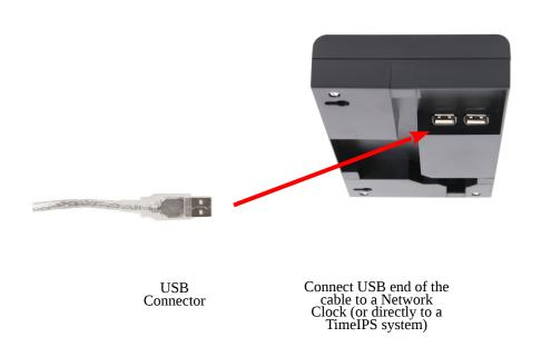
The USB connector can be safely connected to TimeIPS without shutting down. If the Hand Punch reader is not recognized, power cycle the TimeIPS Network Clock.
