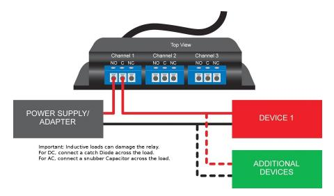
Note: Inductive loads (door locks, other relays, electromechanical bells, etc.) can cause arcing that will damage the relay controller unless a catch diode (for DC) or "snubber" capacitor (for AC or DC) is installed across the load.
