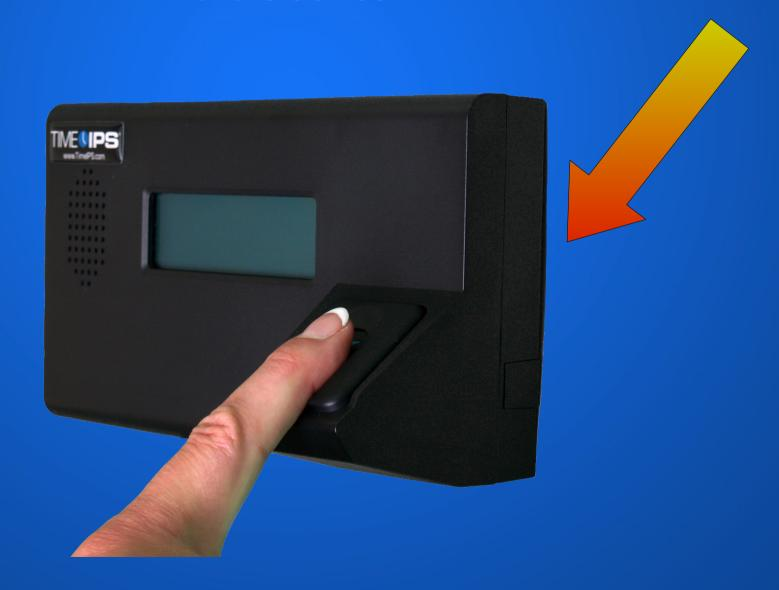
It is **critical** that the finger remain flat and in contact with the device as it slides down the sensor. Don't allow your finger to lift up or down.
