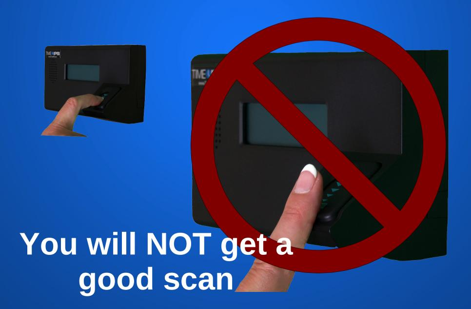
For consistently reliable scans every time, place and pull your finger down the entire length of the device.
