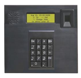
**Optional Installation:** (read thoroughly before proceeding) The keypad can be mounted to the front of the IPS125T. This option requires drilling into the IPS125T housing or the use of hook and loop fastener such as Velcro brand.
