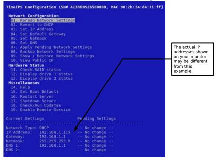
If your DHCP server responds quickly, the table should show an IP address when the boot process is complete. If not, wait a few moments, select Reread Network Settings and press Enter.
