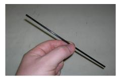
Insert one end of the stir-straw into the fan housing far enough that the fan blades can not spin past it. For some examples of this refer to the following images.
