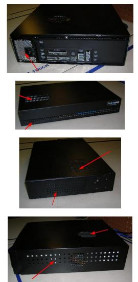
NOTE: Some models of TIMeIPS systems have a fan directly below the vent on the top of the system in the above image. If your TimeIPS system has a fan in this location DO NOT direct compressed air into this vent at this time.
