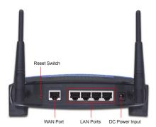
Follow the wiring instructions that came with the router. Connect an Ethernet cable from your Cable/DSL modem to the port marked Internet or WAN on the router. Connect another Ethernet cable from your PC/Laptop to one of the four LAN ports on the router (labeled 1-4).
